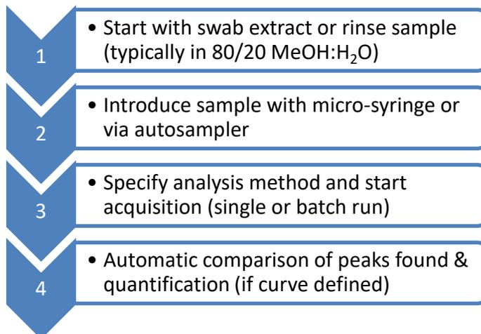
**Fig. 4 Sample analysis workflow with automatic quantification of API/detergents found**
