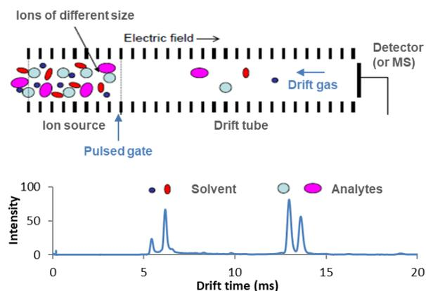
**Fig. 1 Working principle of HPIMS**
