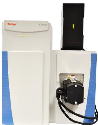
Fig. 8 MA3100 mounted on a Thermo Orbitrap
