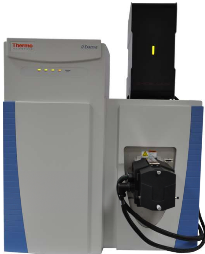
Fig. 1 MA3100 IMS analyzer and control electronics shown interfaced with a Q Exactive™ orbitrap MS. Ion mobility devices from Excellims are now available for a range of Thermo Scientific™ trap-based instruments.
