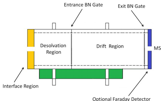
**Fig. 2** Representation of the dual gate ion mobility module indicating interface region, desolvation region, ion gate #1, drift region, ion gate #2, optional Faraday plate detector, and ion trap interface. Coordinated dual BN gate system selects sections of drift time for entrance into the mass spectrometer.
