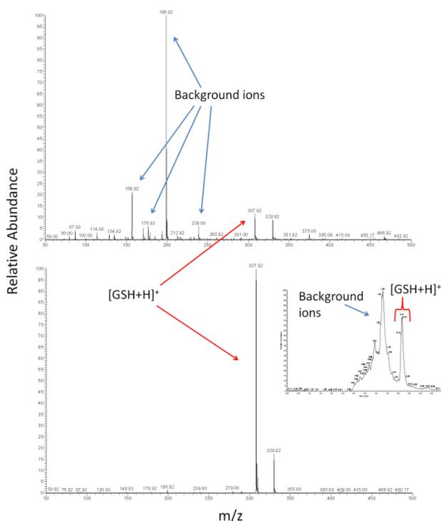
**Fig. 6** Presence of unwanted background ions co-populating trap with GSH (top), and mass spectrum following removal of background ions by operating in “gated” mode, only allowing  $[GSH+H]^+$  to accumulate in the ion trap (bottom). [Inset displays initial IMS scan used to identify drift times of background ions for exclusion].
