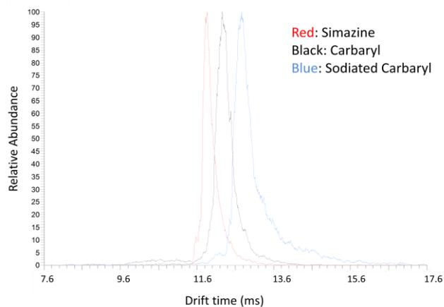
**Fig. 5** IMS “scan” mode for (A) Lys-[Des-Arg9]-Bradykinin + [Val5] Angiotensin II ( $m/z$ : 517) and (B) simazine + carbaryl ( $m/z$ : 202). Note: separation of sodium or similar adducts can result in improved quantitative accuracy.
