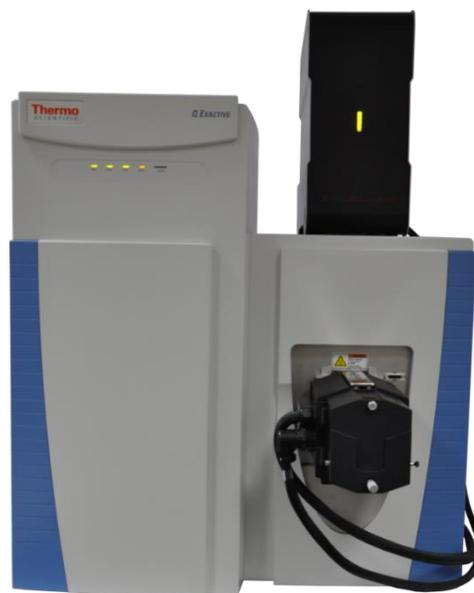
**Fig. 1** MA3100 IMS analyzer and control electronics shown on a Q Exactive™ Orbitrap MS.
