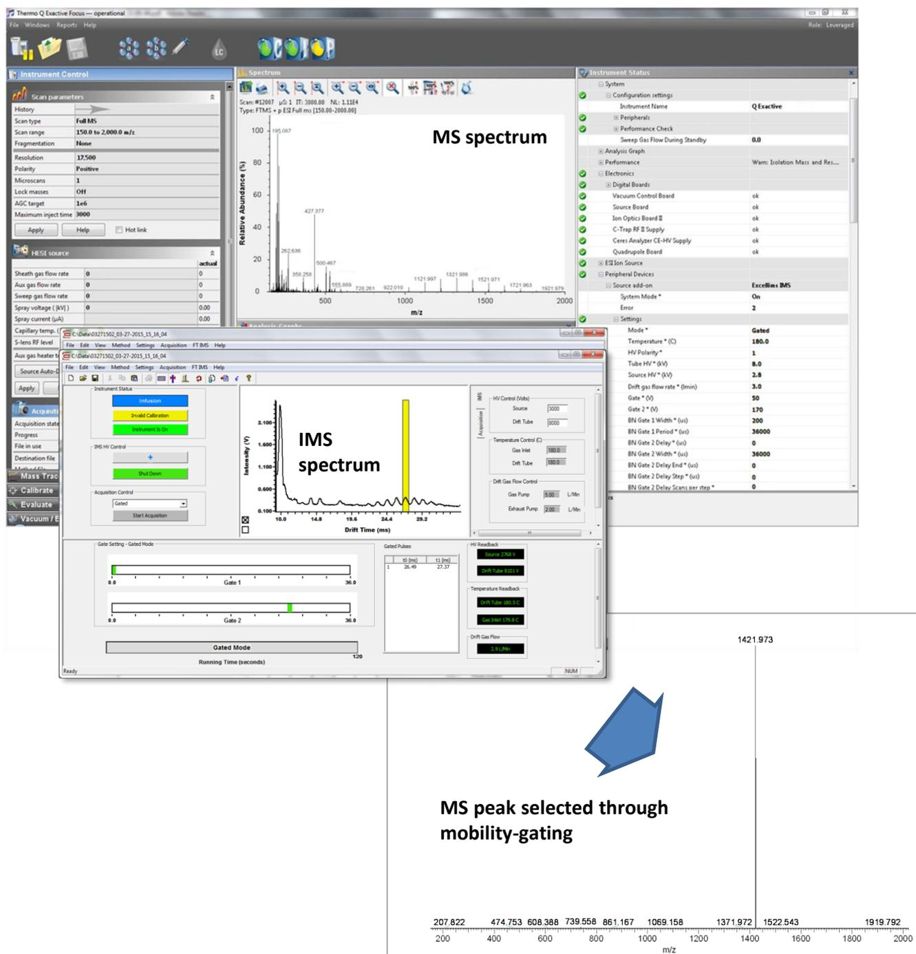
**Fig. 3** Illustration of the MA3100 operating modes: the Tune window (top) shows the entire MS spectrum in OPEN mode while the vision window (middle) displays the corresponding IMS spectrum in FARADAY mode. The yellow marker indicates the selection of one IMS peak selected for further analysis in GATED mode. The GATED mode MS spectrum (bottom) confirms that all but the selected IMS peak have been filtered out successfully.
