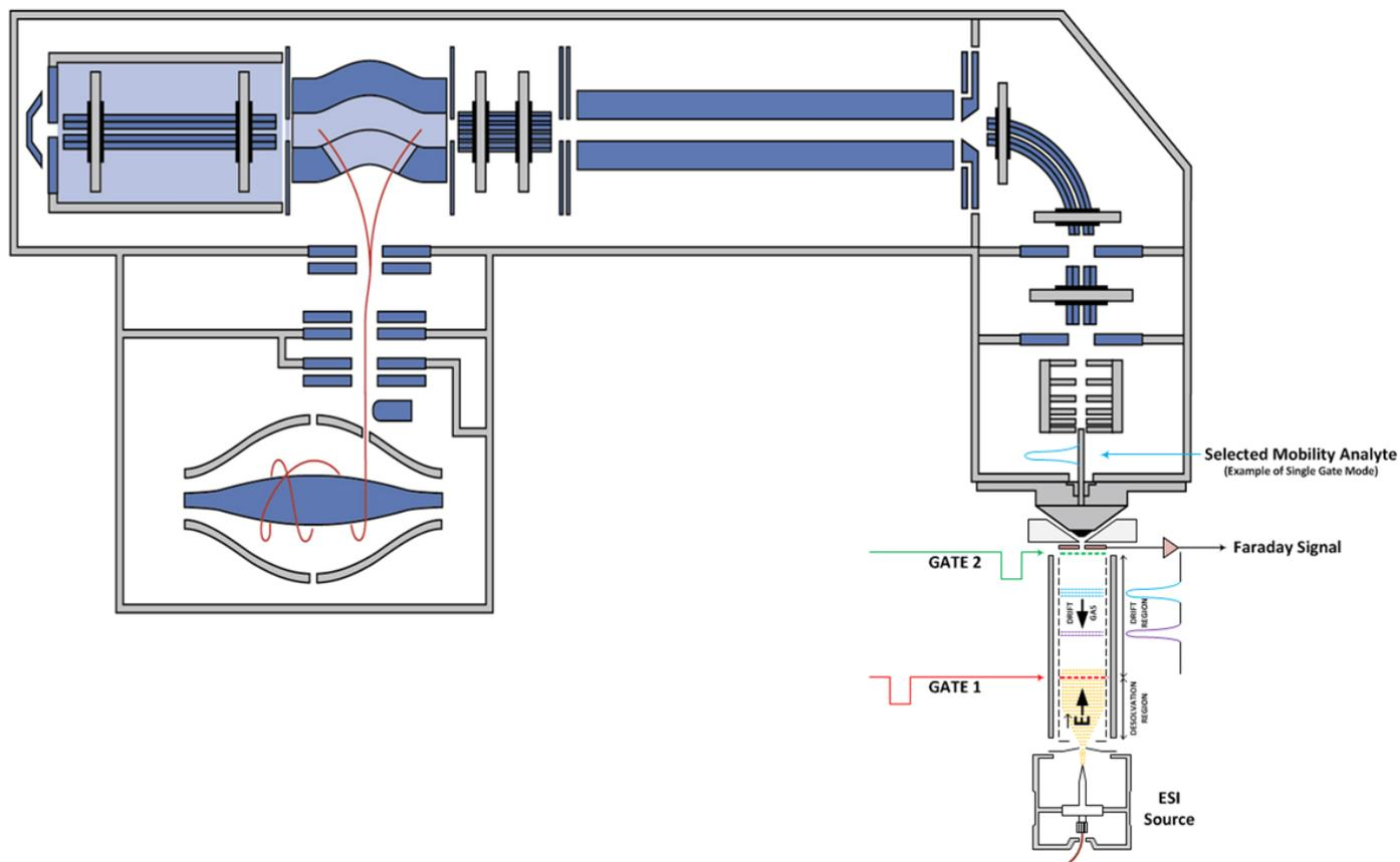
**Fig. 2** The Excellims dual-gate MA3100 is easily coupled with Thermo Fisher Scientific™ mass spectrometers utilizing the Ion Max source design. Four different control modes support simultaneous collection of IMS and MS spectra and selective inclusion or removal of targeted ions based on their drift time.
