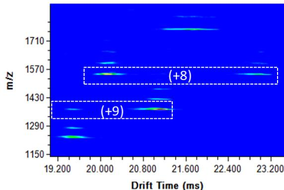
**Fig. 8** Two charge states of ubiquitin (+8 and +9) showing multiple conformers (2D IMS-MS map on Orbitrap)
