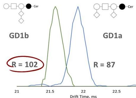
**Fig. 7** Separation of two gangliosides by IMS on the MA3100 with resolving power 80 – 100
