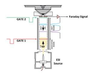
Fig. 9 Diagram showing the dual gates of the MA3100 (for total flexibility in IMS-MS experiments)
